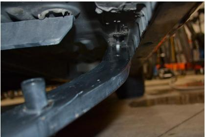
3. Move to the rear and lift the brace, and hand START the two 15mm bolts into the trunk floor reinforcement.
