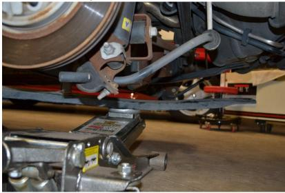
10. Remove the three remaining 15mm bolts on the brace secured by the jack.
