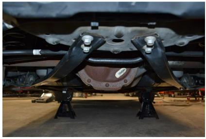
5. The bolts need to be removed in a certain order. Start by removing the two 13mm bolts above the differential (one for each brace). You will need a combination of socket and extensions that are at least 16 inches long to reach them.
