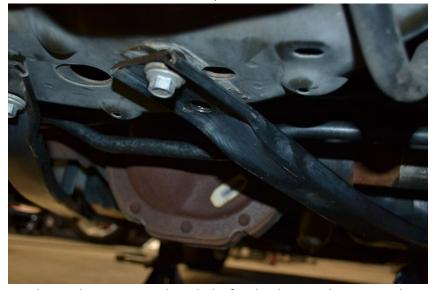
4. Hand start the remaining three bolts for that brace. Please note that middle bolts are coated with bolt sealer/locker that you should reapply.
